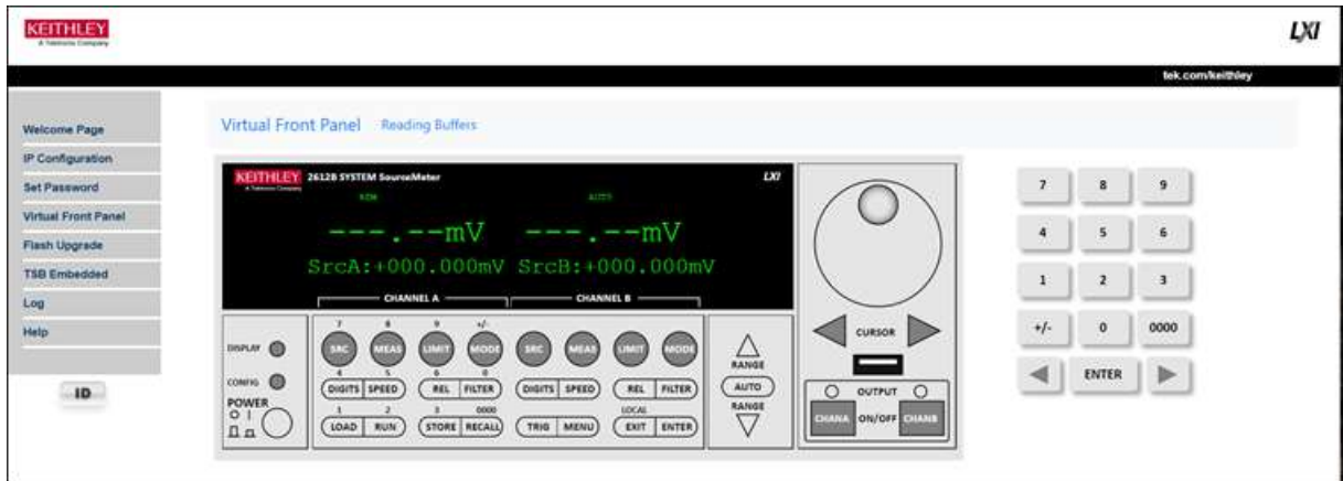
Figure 18: Virtual front panel
