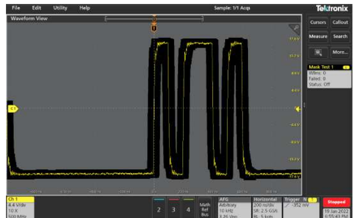
Limit mask test based on golden reference signal
