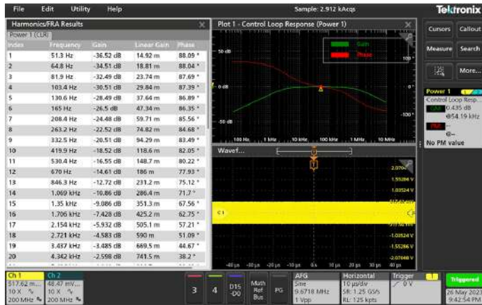
Frequency Response Analysis on the 2 Series MSO.
