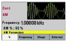
Both models provide AM and FM modulation along with linear/logarithmic sweep and built-in counter capabilities. Internal and external sources can be used for triggering and modulating the signal.
