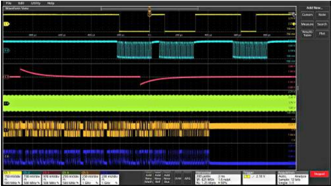
Stacked display mode enables easy visibility of all waveforms while maintaining maximum ADC resolution on each input for the most accurate measurements.
