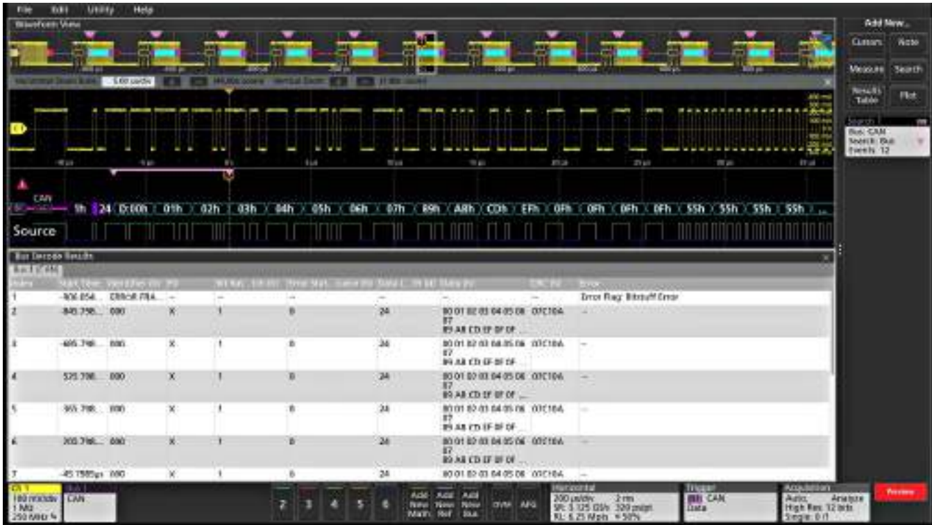
Triggering on a CAN serial bus. A bus waveform provides time-correlated decoded packet content including Start, Arbitration, Control, Data, CRC and ACK while the bus decode table presents all packet content from the entire acquisition.
