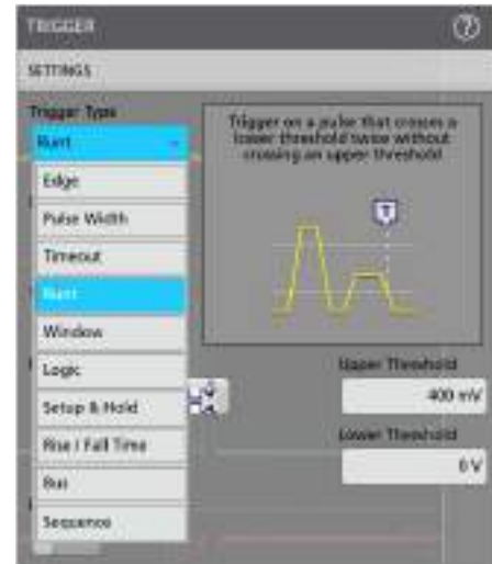
The wide variety of trigger types and context-sensitive help in the trigger menu make it easier than ever to isolate the event of interest.
