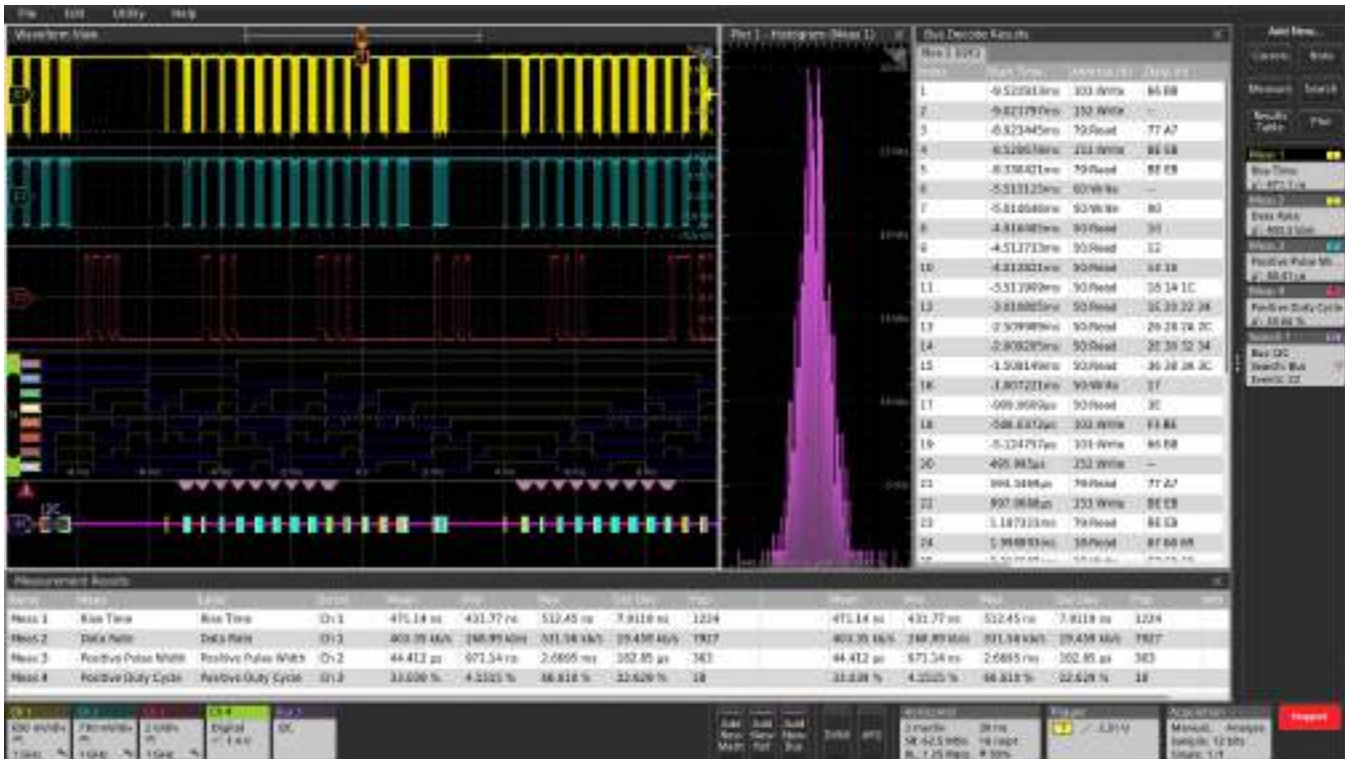
Viewing three analog channels, eight digital channels, a decoded serial bus waveform, decoded serial packet results table, four measurements, a measurement histogram, measurements results table with statistics and a search on serial bus events - simultaneously!
