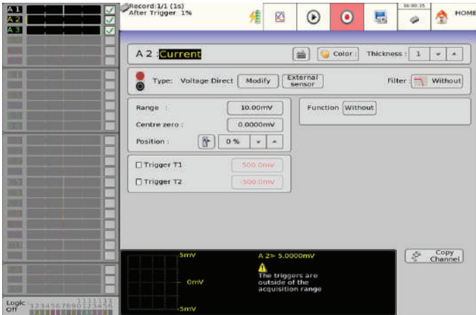
Channel setup displays parameters for up to 12 channels on a single screen
