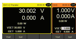
Channel 1+2 parallel view
