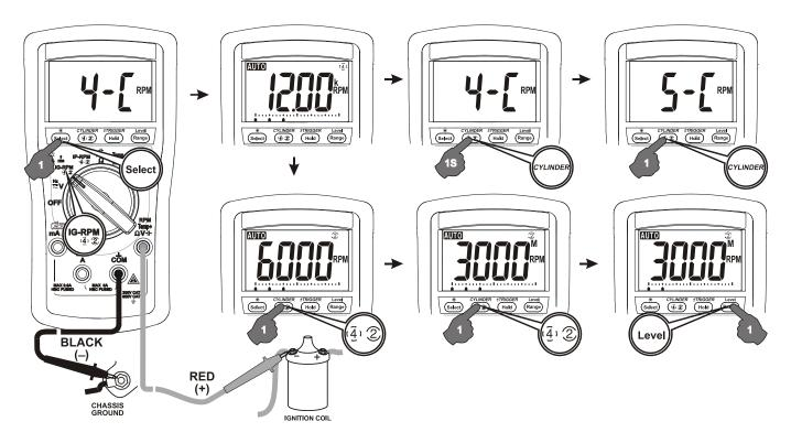
Press 4 button momentarily to select through **RPM**4 for 4-stroke, **RPM**2 for 2-stroke and DIS, and **RPM**2 **M** for special 2-stroke waste ignition engine
