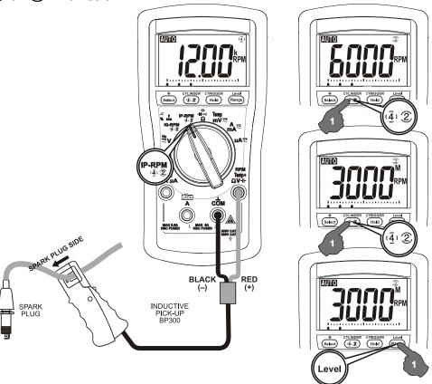
Press (4) button momentarily to select through **RPM**(4) for 4-stroke, **RPM**(2) for 2-stroke and DIS, and **RPM**(2) **M** for special 2-stroke waste ignition engine
