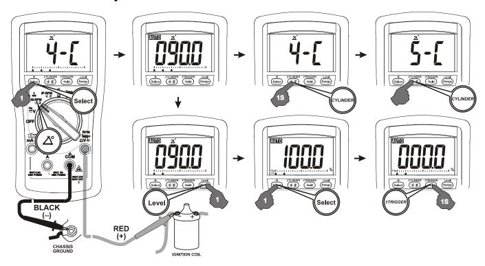
Number of cylinders defaults at 4 cylinders. Press **Cylinder** button for one second or more to display the cylinder setting, and press momentarily again within one second to select the number of cylinders from 1 through 12 to match the engine under test. Adjust the dwell angle according to the procedures outlined in your vehicle service manual. Re-check the timing whenever the dwell angle has been adjusted.
