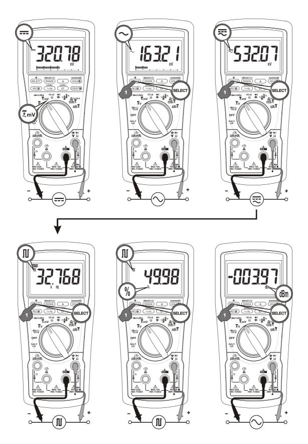
**Note:** In dBm function, power up default reference impedance will be displayed for 1 second before displaying the dBm readings. Press  $dBm-\Omega$  (RANGE) button momentary to select different reference impedance of 4, 8, 16, 32, 50, 75, 93, 110, 125, 135, 150, 200, 250, 300, 500, 600, 800, 900, 1000, up to  $1200\Omega$ . Last selection will be saved as power up default for repeat measurement convenience.
