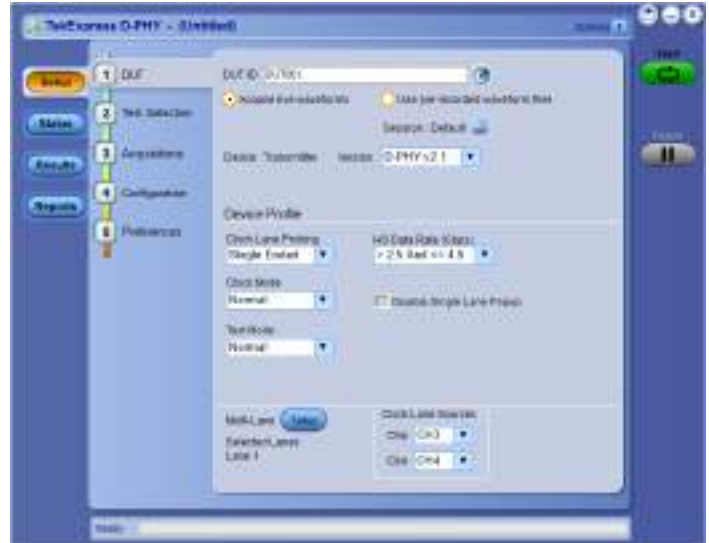
TekExpress D-PHY (Options DPHY12, DPHY21) - TekExpress® D-PHY application offers a complete physical layer test solution for transmitter conformance and characterization as defined in the MIPI D-PHY version 1.2 and version 2.1 specifications. The automated test solution provides an easy way to test, debug and characterize the electrical and timing measurements of D-PHY data links.
