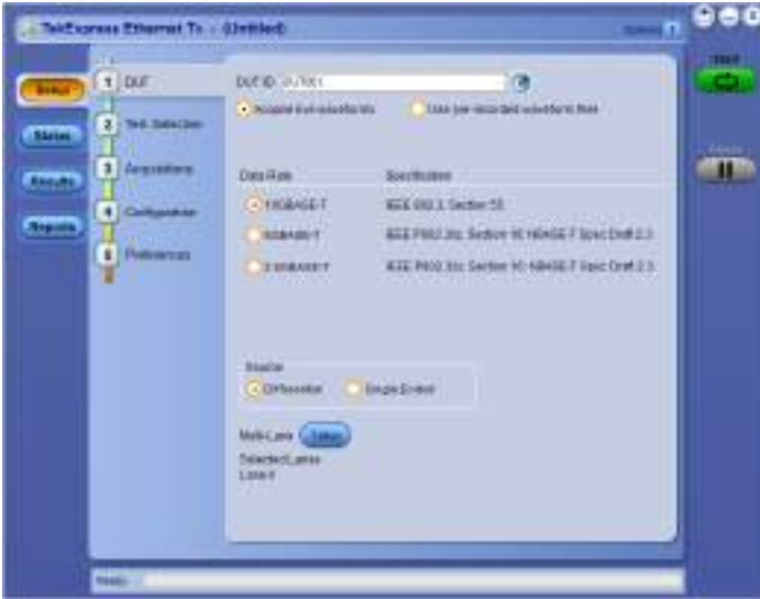
TekExpress Ethernet Tx (Options NBASE-T, XGBT2) – Automates 10GBASE-T, NBASE-T, and IEEE802.3bz (2.5G/5G) physical medium attachment (PMA) and physical-layer (PHY) electrical testing to provide a fast and accurate way of testing your Ethernet designs.
