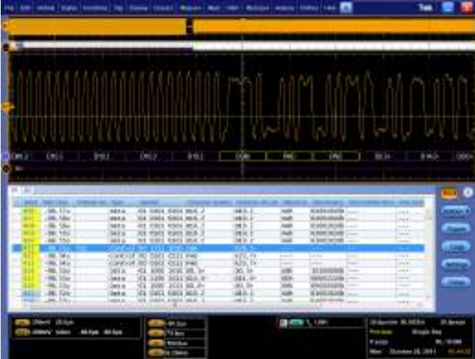
Protocol and Electrical Views of an HSS Bus. The data in the results table and the acquired waveform are time correlated, enhancing the ability to identify possible causes of protocol errors due to electrical signaling.
