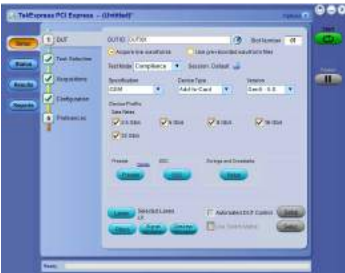
TekExpress® PCI Express Gen 1/2/3/4/5/6 Automated Test Software (Options PCE3, PCE4, PCE5, PCE6) - Provides the most comprehensive solution for PCI Express transmitter compliance testing from legacy Gen1 to most recent Gen6 BASE (as of Oct 2022). Covering troubleshooting and validation of PCI Express devices corresponding to the PCI-SIG specifications. The application automates selection of appropriate fixture de-embed, reference channel emulation filters, and measurement selections based on test type, device data rate, transmitter equalization, link width, and selected probes. TekExpress includes compliance automation solution that integrates the PCI-SIG's Sigtest test software with Tektronix DPOJET-based PCI Express Jitter and Eye Diagram, SDLA Serial Data Link Analysis Visualizer analysis tools for debug, as well as PAMJET for Gen6 PAM-4 modulation analysis. Results are presented in a comprehensive HTML format for engineering test documentation.
