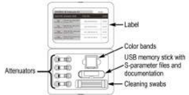
DPO7RFK1-1.85 mm characterized attenuator kit.
