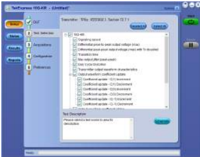
10GBASE-KR/KR4 Compliance and Debug Solution (Option 10G-KR) - Automated compliance measurements for IEEE 802.3ap-2007 specifications. This option includes an automated compliance solution and debugging with DPOJET. The automated test setup measures transmitter equalization levels generating 12 results for each tap and 120 results for 9 different measurements in approximately 15 minutes.
