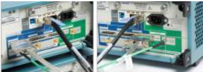
UltraSync connection on instrument with Master role
