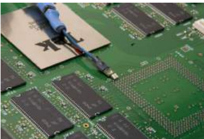
The low-cost solder tips available for the P7500 TriMode probes allow quick connection so moving the probe to various solder points is fast and easy.
