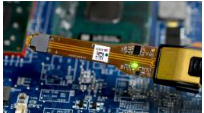
P77STFLXA solder down, flex circuit accessory with an active buffer amplifier on its tip provides up to 20 GHz bandwidth.
