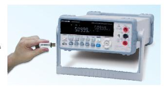
The USB storage function allows each flash drive to establish 100 folders (GW000  $\sim$  GW099). Each folder has a capacity of saving 5,000,000 data files (which are divided into 100 sub-file names, therefore, each sub-file name can save 50,000 data files. Take folder GW000 as an example, internal file names are GW000 $_{\rm C}$ 00  $\sim$  GW00 $_{\rm C}$ 99). The storage format is CSV, which can open files and conduct file analysis by existing tools. (such as Microsoft Excel)
