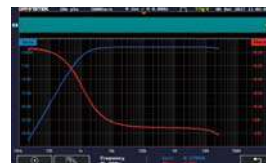
FRA of RC high-pass filter
