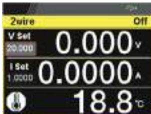
White: Temperature Control on with GTL-205A Connected
