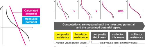
The calculated potential is computed while varying the variables.
