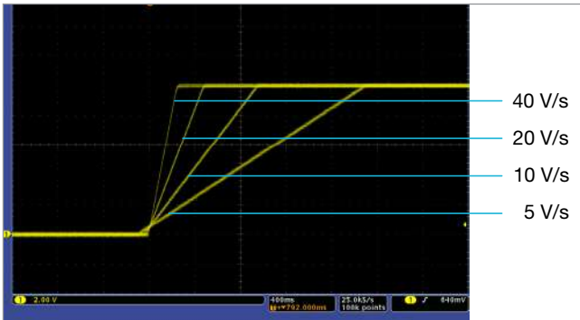
Precisely control voltage rise time with the variable slew rate control.
