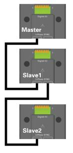
The TL983P adapters connect to the Digital I/O connector on the rear of the AC source. Standard RJ45 communication cables connect each adapter to route the 3-phase synchronization signal from the master to the slave units.
