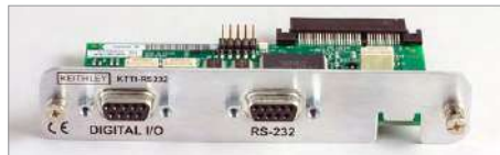
KTTI-RS232 RS-232 interface with 6 digital I/O ports.
