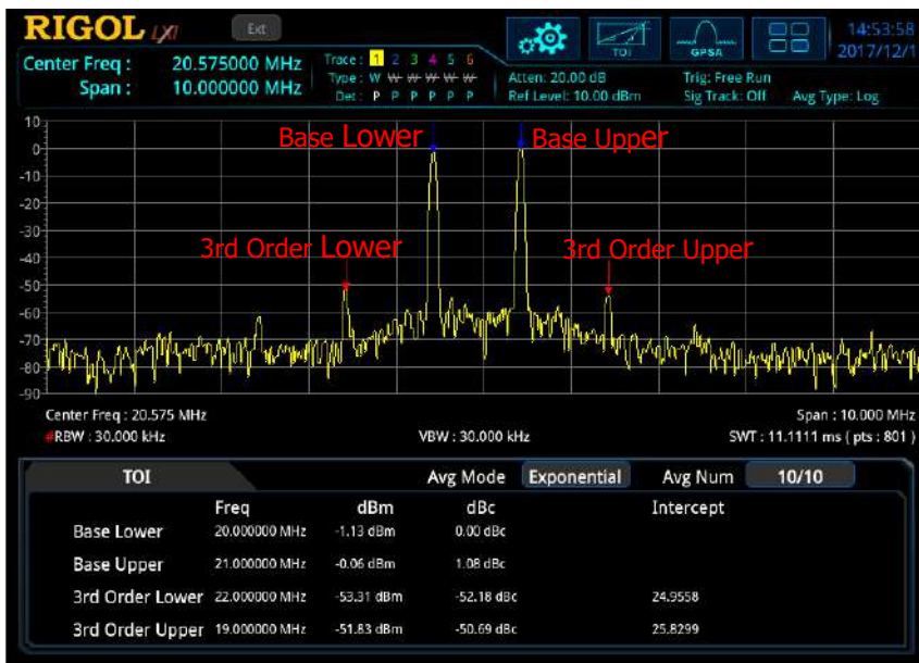
Figure 2-12 TOI Measurement Interface
