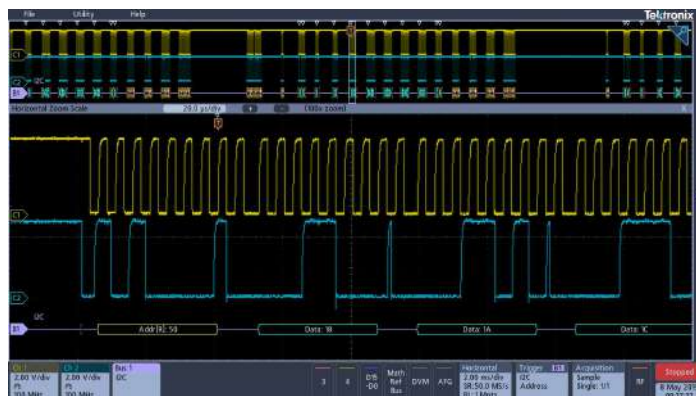
Triggering on a specific address and data packet going across an I 2 C bus. The yellow waveform is clock and the blue waveform is the data. A bus waveform provides decoded packet content including Start, Address, Read/Write, Data, and Stop.
