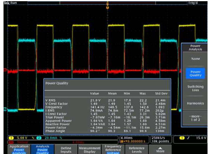
Power quality measurement. Automated power measurements enable quick and accurate analysis of common power parameters.
