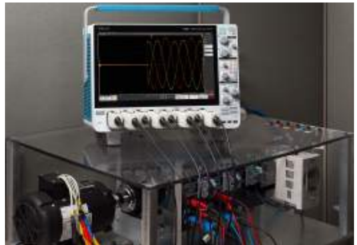
Voltage measurements on a three-phase motor showing the three-phase input voltages after start-up.
