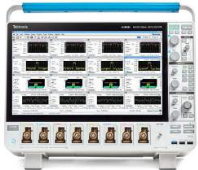
MSO68 showing SignalVu-PC multi-channel VSA software running on the instrument
