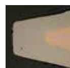
Weller WSW after 10,000 solder cycles
