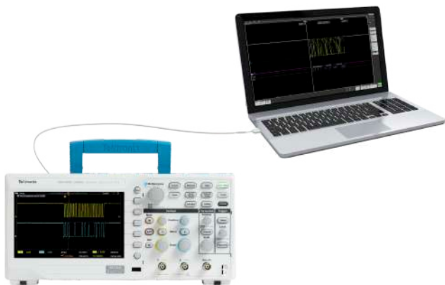
Waveform analysis with TekScope on a PC
