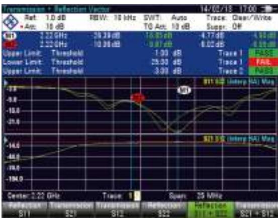
Vector network analysis: Simultaneous display of four S-parameters ( S_{11} , S_{21} , S_{12} , S_{22} )
