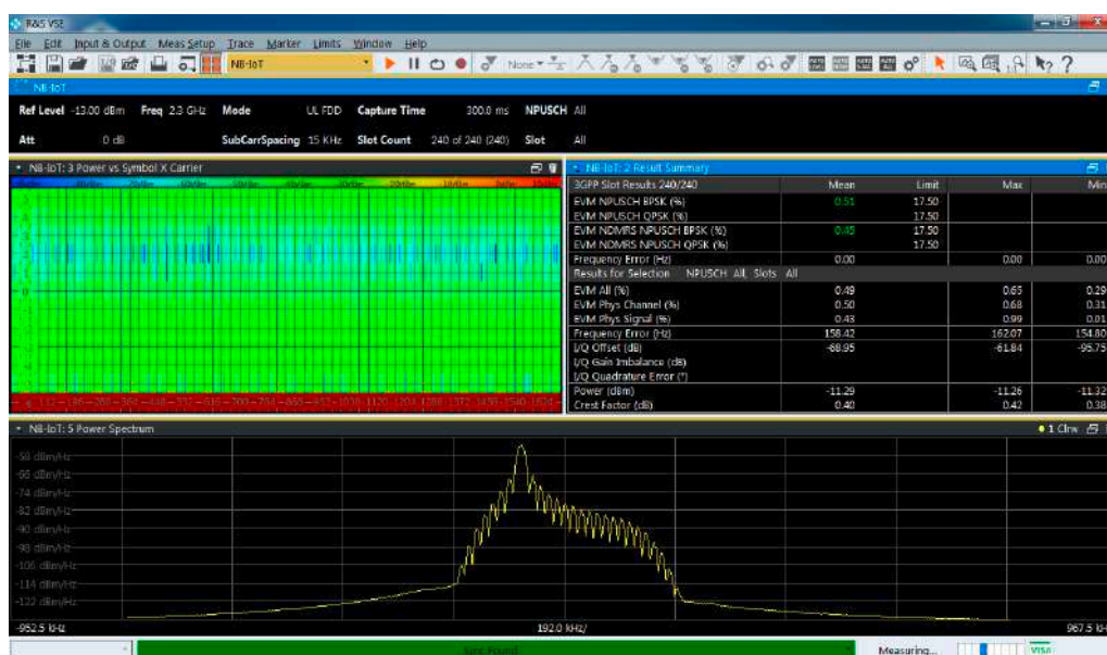
Demodulation and EVM measurement of an NB-IoT UL signal with the R&S®VSE-K106 measurement application
