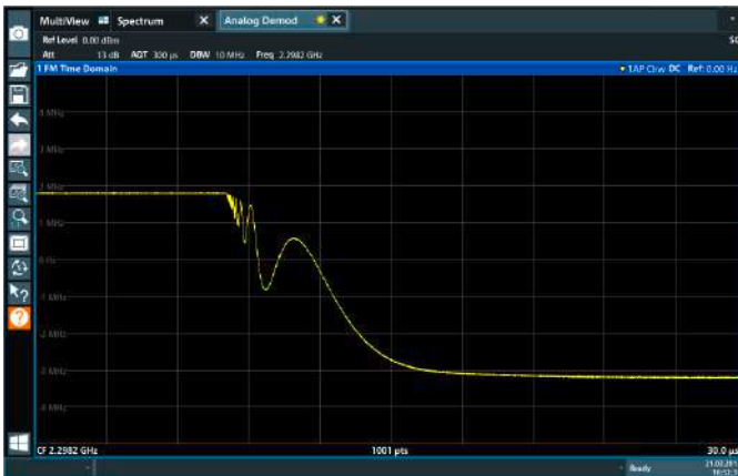
Frequency settling behavior of an oscillator
