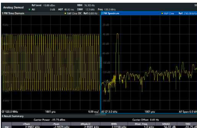
Display of the modulating signal and its spectrum together with peak and RMS deviation
