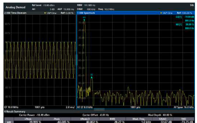
THD measurement on an amplitude modulated signal: the first harmonic of the modulation signal is well suppressed by 74 dB
