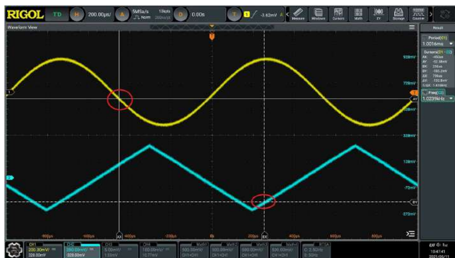
Figure 10.14 Track Measurement (after Horizontal Expansion)
