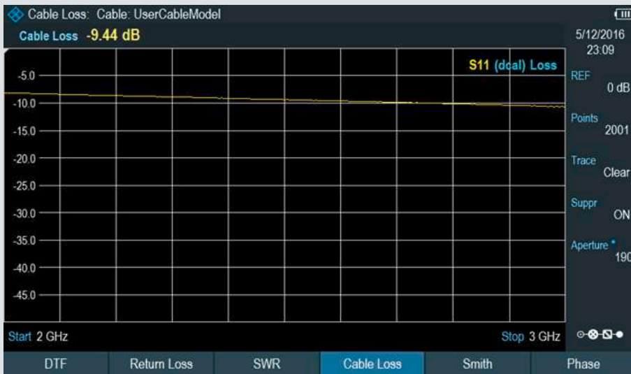
One-port cable loss measurement
