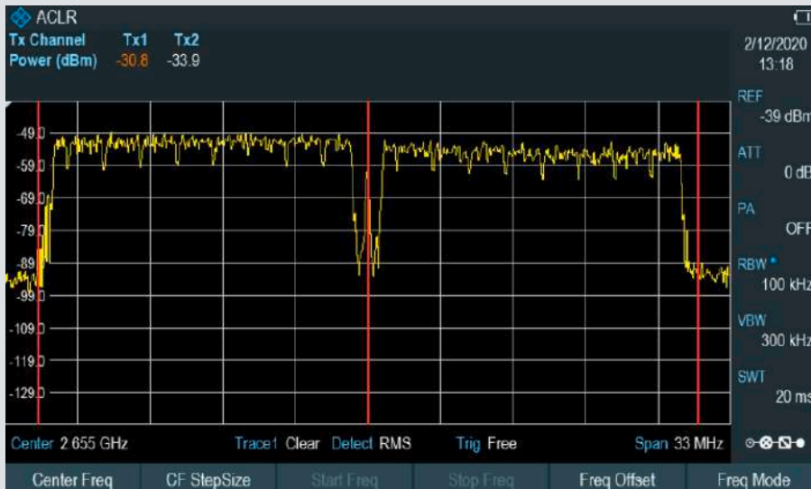
Gated trigger in ACLR mode with advanced the R&S®ZPH-K57 advanced gated trigger measurements option
