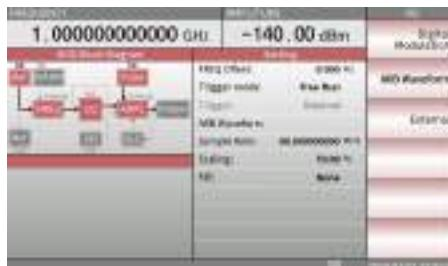
8. To select external waveform modulation, press the F3 key.
