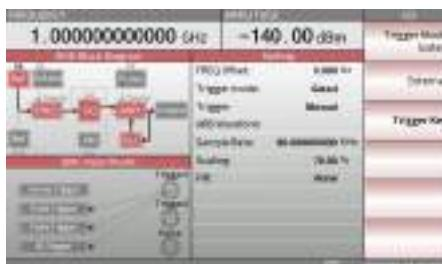
2. Set trigger mode. Press the F1 key to change trigger mode.
