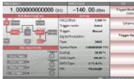
6. To select the External trigger, press the F2 key.
