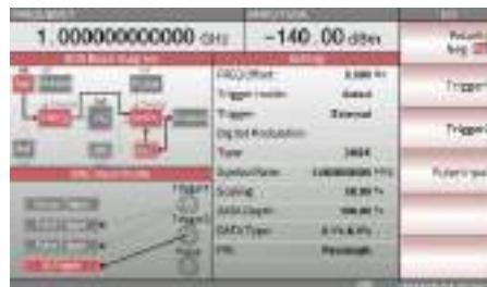
7. Press the F1 key to select polarity. There are polarities positive and negative. You can see the difference from the BNC input route diagram.
