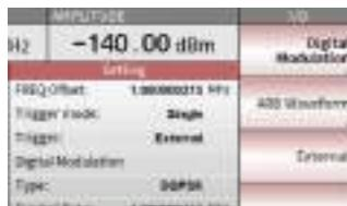
6. To select digital modulation, press the F1 key. Then you will see the further option about digital modulation appears as shown in the figure below. For further digital modulation settings, please refer to page 113.
