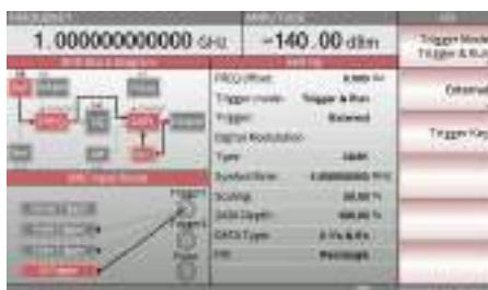
5. To select the Manual trigger, press the F3 key.
