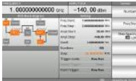
9. Press the F6 (More) and toggle the F3 keys to select step spacing in MHz or percentage.
