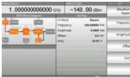
2. Press the F1 key to change the waveform when the LF output is activated.
