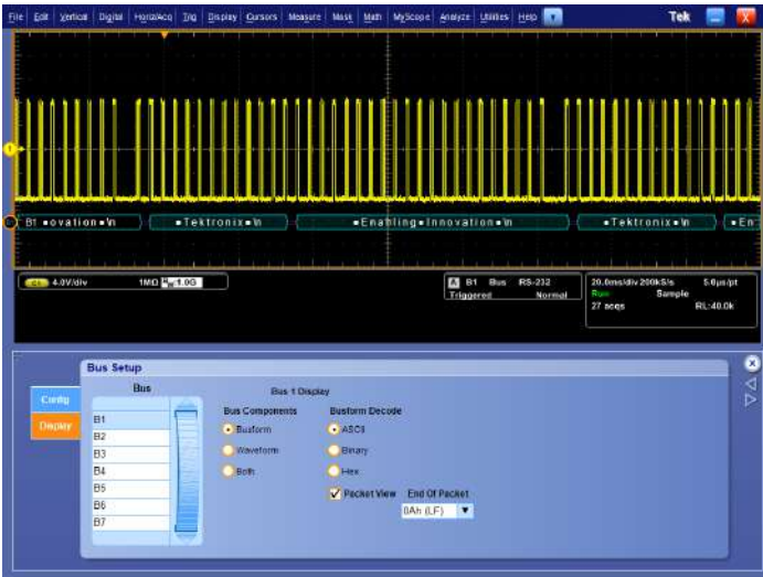
Packet View display of decoded RS-232 messages.
