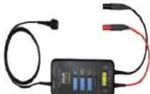
PHA0150  | High-voltage Differential Probe | <ul style="list-style-type: none"> <li>• BW: DC to 70 MHz</li> <li>• Max. voltage <math>\leq</math> 1500 Vpp</li> <li>• Compatibility: All models of RIGOL's digital oscilloscopes</li> </ul>                                                                            |
