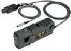
RP1005C   | Current Probe        | <ul style="list-style-type: none"> <li>• BW: DC to 10 MHz</li> <li>• Maximum Input AC P-P: 300 A (non-continuous), 500 A (@pulse width <math>\leq</math> 30 us)</li> <li>• AC RMS: 150 A</li> <li>• Compatibility: All models of RIGOL's digital oscilloscopes</li> <li>• Required to order RP1000P power supply.</li> </ul> |
