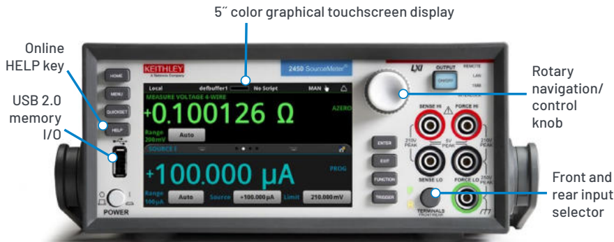
2450 front panel with high-resolution, capacitive touchscreen.
