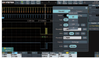
Standard 5 Serial Bus Trigger & Decode Functions: RS232/UART, I 2 C, SPI, CAN, or LIN
