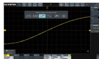
Detecting Square or Pulse Waves, the Second-level Menu Optimizes Pulse Width and Edge Timing Measurements
