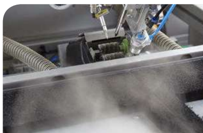
Safety cover fully encloses the integrated fume extraction system, protecting the user, workpiece, and equipment
